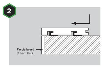
Insert the *HD Deck Dual*® bullnose deck board over the clips and push it forward. Secure in place with Universal Clips as required.
