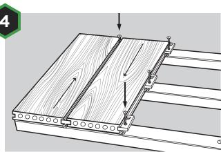
Take the next piece of deck and securely push into the Universal Clips. Now nip the screw to secure the Universal Clip against the board. **Do not over tighten**. Now repeat steps 3 and 4 to cover the deck, using one Universal Clip and screw on every joist. For a more natural finish, we recommend **alternating the direction of the wood grain** when installing the boards. If using the bullnose board, use this as your starting point.
